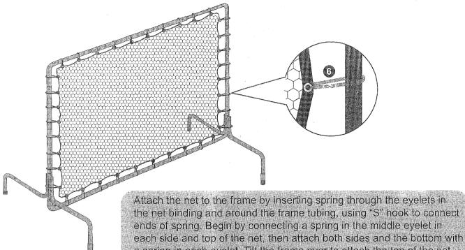
a spring in each eyelet. Tilt the frame over to attach the top of the net. If your net hangs too loosely on the frame, substitute 3510W Shorter Springs and "S" hooks on one side (left or right) and top (or bottom). This will make net more taut.
