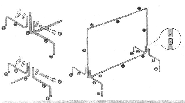
Using part list, identify each tubular part & lay out as shown. Assemble the frame as indicated in the drawing. Attach rubber leg caps on the bottom of the stand legs. For tilt adjustment to practice "lobs", remove two rubber caps and install the extension.
